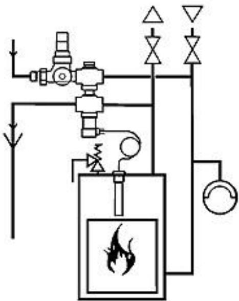
Thermal protection of the installation is used to protect solid fuel boilers in heating installations equipped with thermostatic valves in accordance with the Polish Standard PN-EN303-5. It is particularly recommended for boilers that are not equipped with a cooling exchanger.
