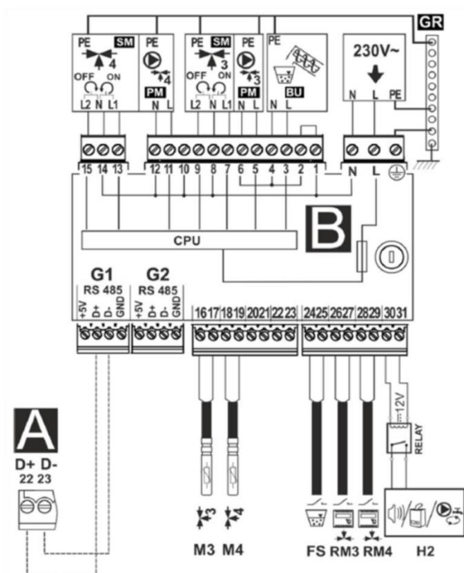
Electrical connection diagram - additional module B, where:
