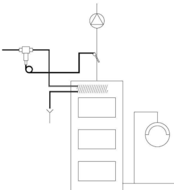
In solutions with a safety coil built into the boiler, e.g. thermal protection is used.
