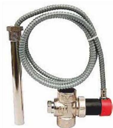
The emergency extinguishing device, protecting against fuel ignition in the tank, can also be connected to the water supply system and when the set temperature is exceeded, the extinguishing device opens the water valve and operates independently of the electrical power supply.
