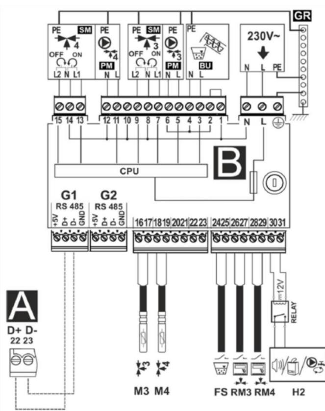
Electrical connection diagram - additional module B, where:
